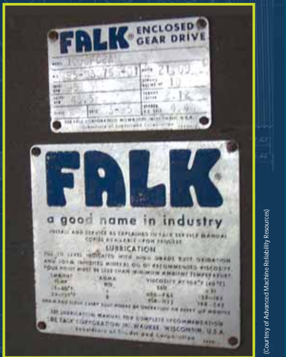
Figure 11. Gear drive faceplate label showing viscosity parameters
