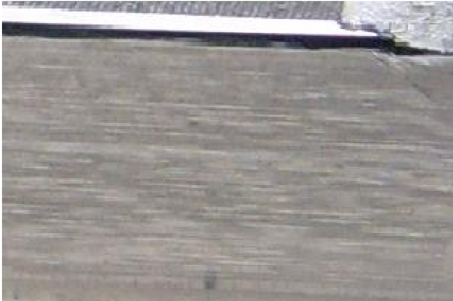
Figure 6 | Wind turbine gear drive flank after surface conditioning.
