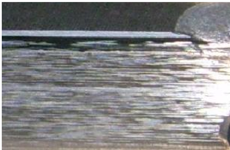
Figure 3 | Surface of a rough gear flank from a wind turbine drive.
