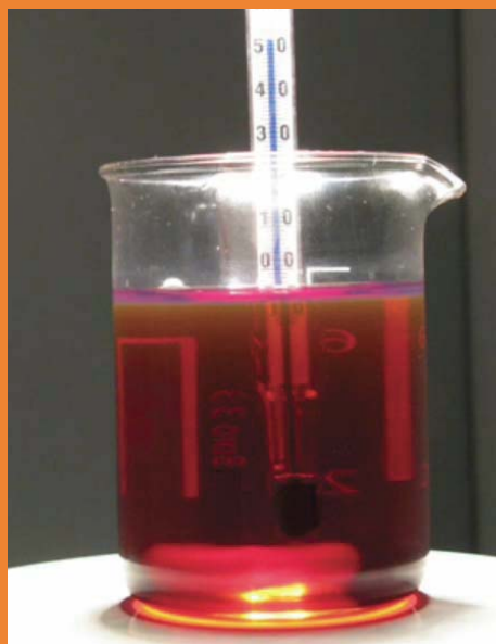
Figure 4 | At 50 C, the oil instantly becomes clear and bright as the degradation products solubilize. [Courtesy of Ansaldo Thomassen, The Netherlands]
