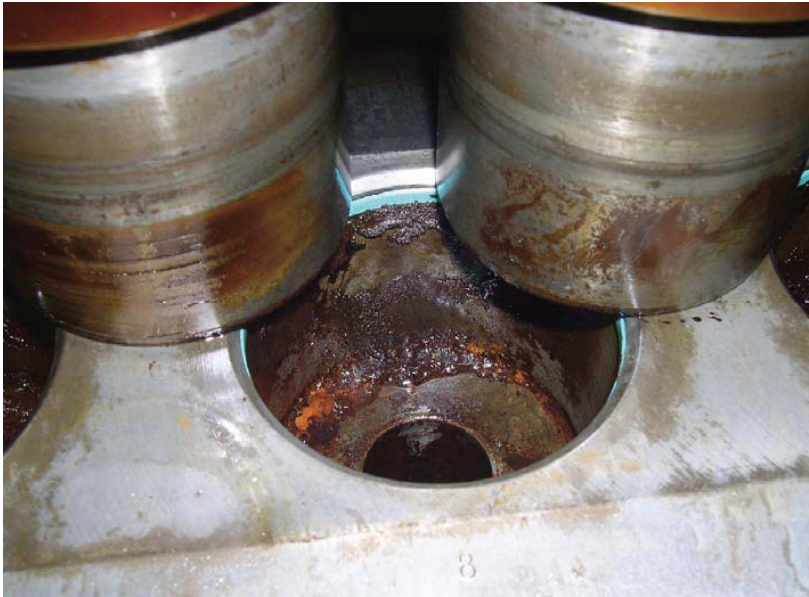
Figure 1 | Deposits in a sensitive paper machine can impact the quality of the finished paper product.
