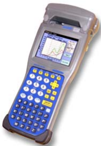
Figure 5 | The RULER instrument for antioxidant measurement [Courtesy of Fluitec].
