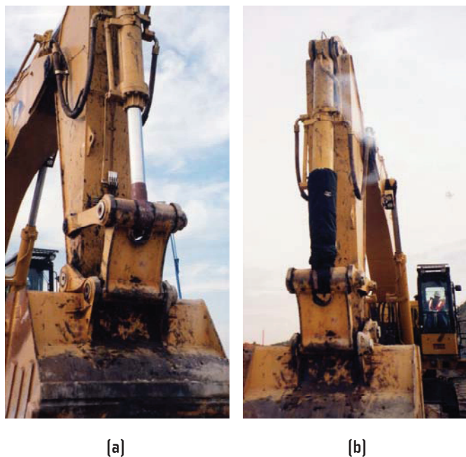
Figure 8 | Before and after the seal savor is placed in service. [Courtesy of Fluid Control Services, Inc.]
