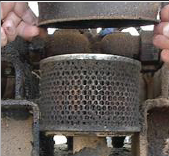
Figure 5 | A chrome OEM breather vent and the upgrade desiccant element and mounting base.
