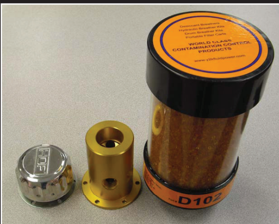
Figure 5 | A chrome OEM breather vent and the upgrade desiccant element and mounting base.
