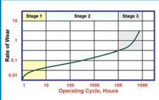
Proper lubricant selection can slow the onset of progressive wear (Stage 3) and also help dampen the shock-loading forces that lead to cyclic fatigue failure. The type of lubricant selected is highly dependent on the chain application. Chain lubricants are category of products with a significant degree of specialization and sophistication, particularly for elevated temperature application.
